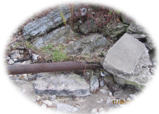
Four inch gas pipe which was ripped from the river bed by the rail car carrier Maitland # 1 as it remains on Brown's Point today.
